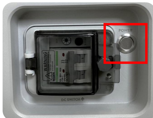
Figure 19: Switching off the battery.
