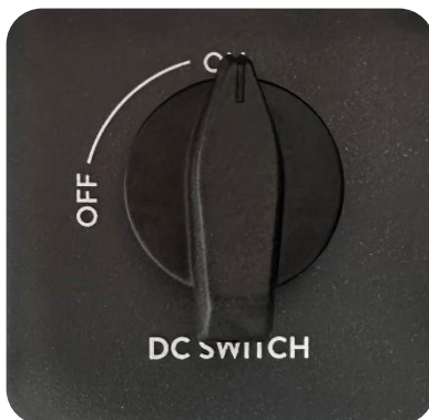
Figure 17: Deactivation of the photovoltaic direct current supply_1.1
