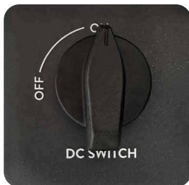
Figure 17: Deactivation of the photovoltaic direct current supply_1.1
