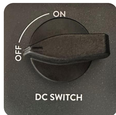
Figure 18: Deactivation of the photovoltaic direct current supply_1.1
