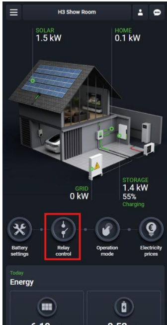
Figure 22: Menu Item Relay Control
